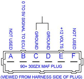
\*Due to the variations of Nissan wiring between models, this may not be the correct Nissan MAF sensor pins for the model you are working on. You must confirm that 300ZX pin "E" is connected to 12v+. 300ZX pins "C" and "D" are connected to the Nissan ground wire. 300ZX pin "B" must be connected to the Nissan 0-5V MAF signal wire.
